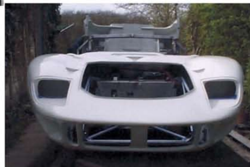
Rear bulkhead rollover frame and rear subframe in place, oil and cooling pipes in central tunnel
