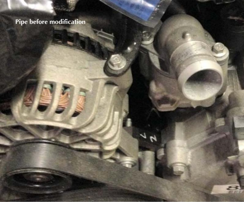
had a problem with the exit of one of the water pipes from the engine; this came from the top and was butting up against the rear bulkhead. Mick said he would alter it to go in a different direction and, as you can see from the pictures, he did a super job - welding in aluminium isn't easy.
